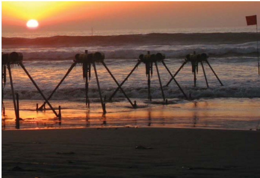
Huge tripods position acoustic Doppler velocimeters (ADVs) at precise heights in the swash zone above San Diego, Calif. in Woods Hole Oceanographic Institution researcher Britt Raubenheimer's study of current and sediment movement.
